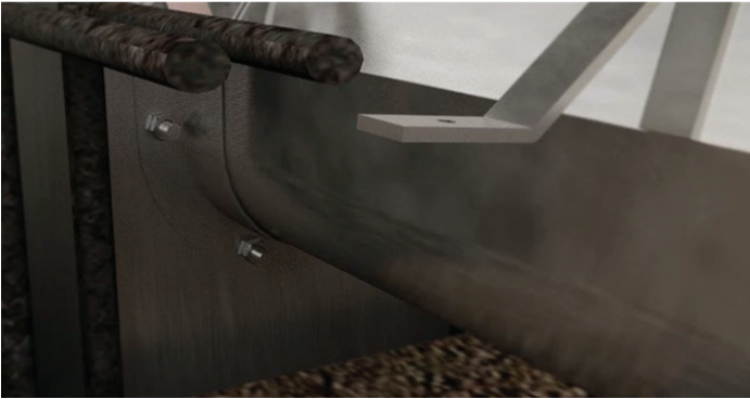
DEEPEST SECTION OF DRAIN AND CATCH BASIN CONNECTED TOGETHER
